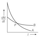
We know that  $\left(\frac{dN}{dt}\right) \propto$ ,  $\lambda$ , at any instant of time hence we can say that  $\lambda_A > \lambda_B$ . At point *P* shown in the diagram the two curve intersect.
