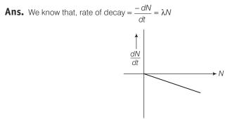
where decay constant ( $\lambda$ ) is constant for a given radioactive material. Therefore, graph between *N* and  $\frac{dN}{dt}$  is a straight line as shown in the diagram.
